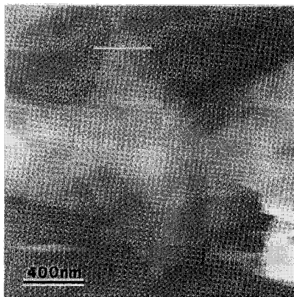
Figure 21. Atomic Force Microscopy-image of single crystals of 2,3-di- O -acetyl-6- O -propanoyl cellulose (Reproduced with permission from Macromolecules 1997 , 30, 6683. Copyright 1997 Am. Chem. Soc.).
